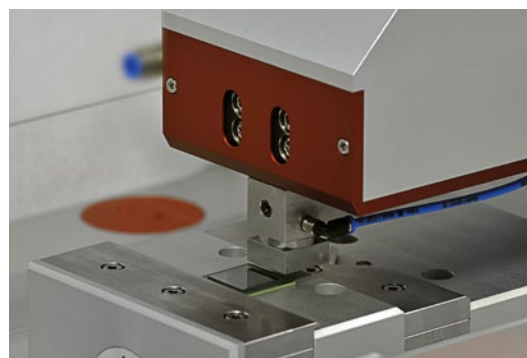
Self aligning shear tool: The application is mounted on a special die shear work holder.
